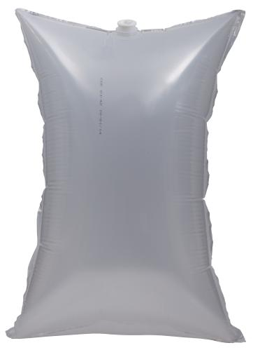
When filled, these industrial tote liners form the shape of a pillow. Pillow-shaped liners are typically constructed with two or three plies of linear low-density polyethylene (LLDPE) and a barrier film when used for aseptic and oxygen-barrier applications. The 55 gallon pillow style liner with a 2" fill fitment works for all types of 55 gallon drums.
