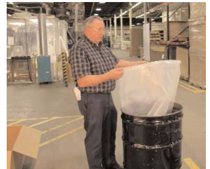
Insert liner into drum.
