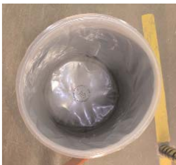
Sides of liner should be smooth and CDF logo should be centered in drum.
