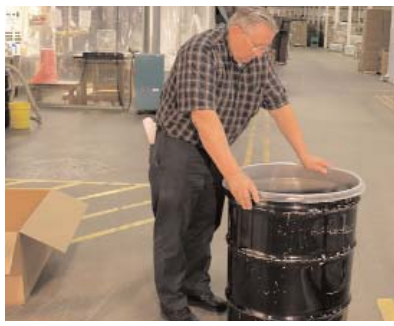
Lightly push the top of the liner down.
