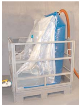
Air-assist liner will begin to stand as more product is forced out.
