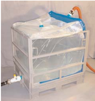
Attach dispense attachment and air-assist attachment. Tote is ready for dispense.
