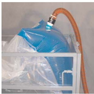
Detail of air-assist liner inflating.
