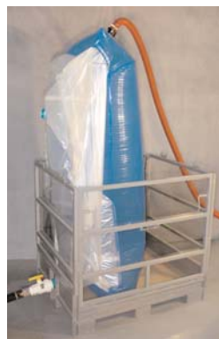
Air-assist liner evacuates product more completely than gravity flow.
