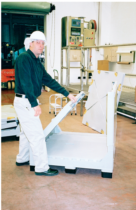
Wild Flavors' operations manager Peter Kindzierski demonstrates quick setup of the returnable bulk container, above, which arrives collapsed for easy shipment, below.
